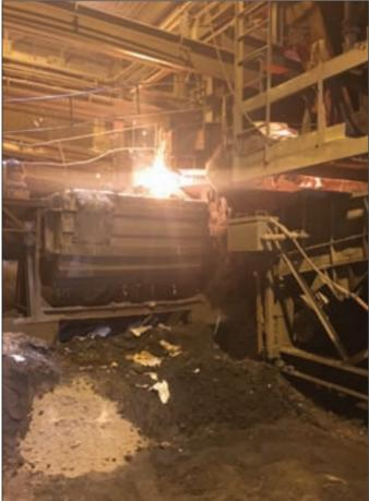
Molten cast iron from furnace being poured into ladle
