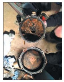
**Photo 1**: What a mess! This old float assembly and housing was packed with mud and sediment and should have been scrapped years ago.
