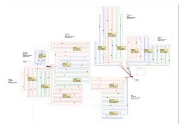
from your favorite tubing manufacturer to create material lists. This program can create scaled drawing outputs set to whatever scale and paper size you desire. An example of a LoopCAD drawing is shown in Figure 2 to the left.
